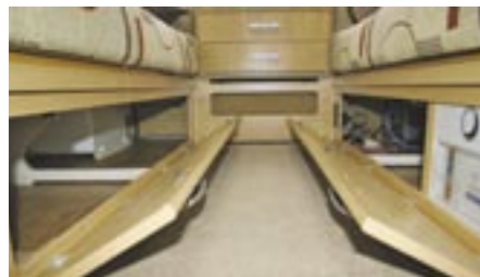
There is a risk these doors could get broken; they would be better if they dropped flat like the Sprite's
